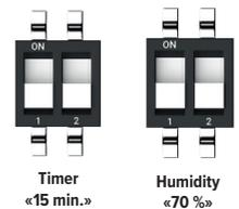
The fan will automatically turn on when the built-in humidity sensor detects its excess of 70% (see SECTION 1) and will work until the humidity sensor detects its decrease to 70% and below (see SECTION 1). After that, the fan will work for 15 minutes (see SECTION 2) and turn off.
