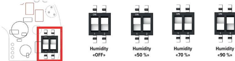
If the humidity sensor is turned off, the fan does not work automatically. The fan will turn on and operate when the power is on.
